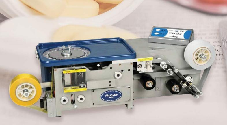
A high quality, compact, fast and efficient unit dose packaging machine for hospitals, long-term care facilities or manufacturing environments. The Cadet Vantage packages 60 units per minute with the standard 1.56 x 2.00" package size. Variable package sizes can be used as well as complete sensors and thermal transfer printing standard.
