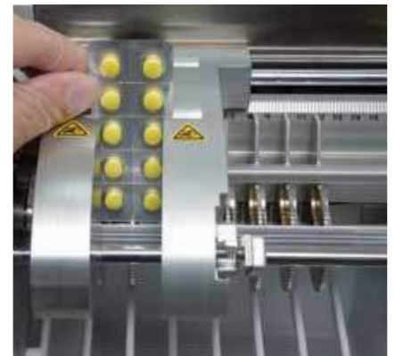
The DB500 can de-blister up to 280 capsules or tablets per minute
